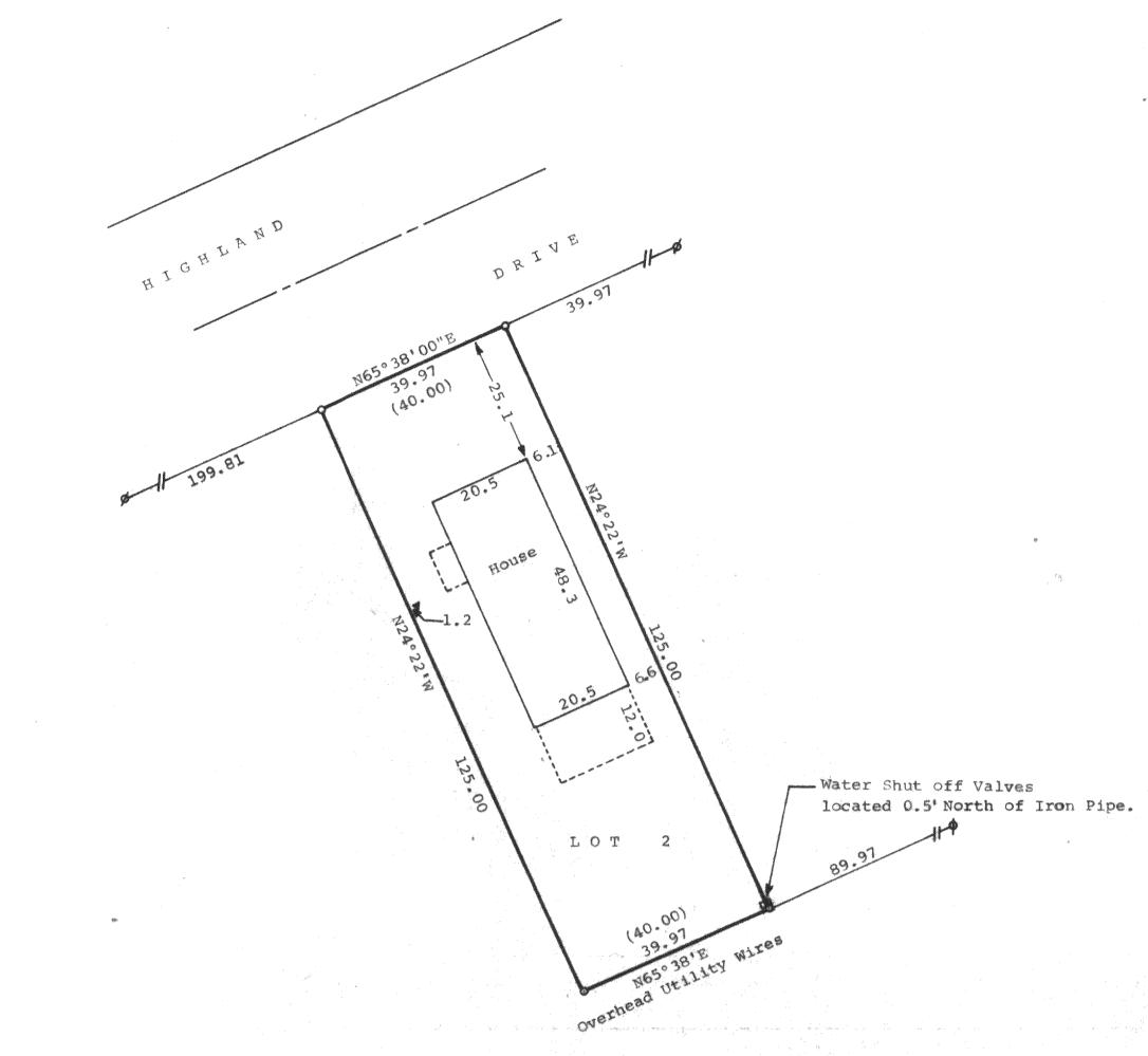
Scale - 1" = 20o = 3/4"x24" Iron Pipe Set  $\emptyset = 3/4$ " Dia. Iron Pipe Found ≠ = ½" Dia. Iron Pipe Found (00.00) = Recorded Distance Bearings are referenced to the Southeasterly line of Highland Drive, Assumed bearing of N65°38'E. Survey Ordered By: The Rauland Agency 607 E. Walworth Ave. Delavan, WI 53115
